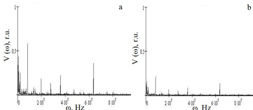
Figure 3.3. – Dependence of the photoacoustic signal from frequency modulation BLB<sub>1</sub> for different  $\rho$ : (a)  $\rho = 10^{-7}$  m; (b)  $\rho = 4 \cdot 10^{-7}$  m
