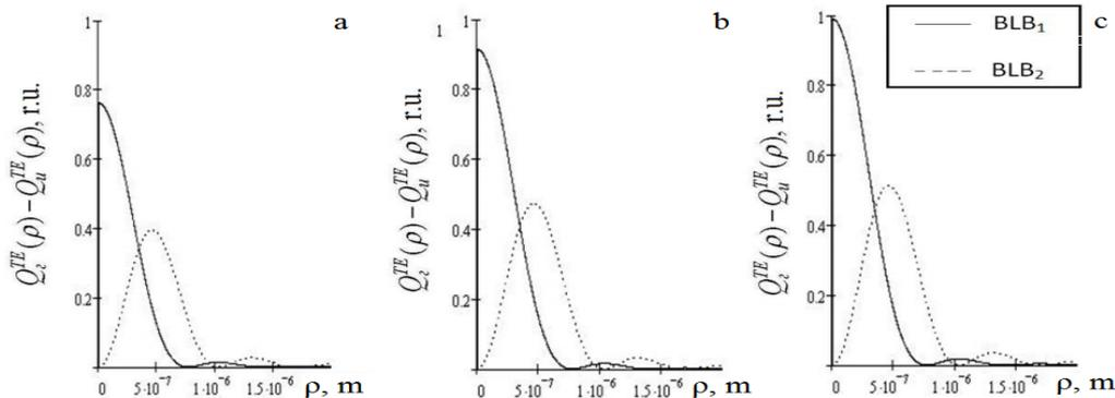
Figure 3.2. – Dependence of the difference of energy dissipation from the  $\rho$  as the parameter of gyrotropy  $\eta_2$   $Q_z^{TE}(\rho)$  and  $Q_u^{TE}(\rho)$ : (a)  $\eta_2 = 10^{-5}$ ; (b)  $\eta_2 = 1.2 \cdot 10^{-5}$ ; (c)  $\eta_2 = 1.3 \cdot 10^{-5}$
